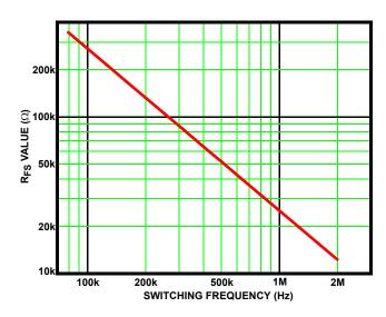
FIGURE 1. SWITCHING FREQUENCY VS. RFS VALUE
