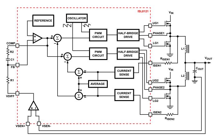
FIGURE 2. SIMPLIFIED BLOCK DIAGRAM OF THE ISL8121 VOLTAGE AND CURRENT CONTROL LOOPS
