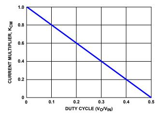
FIGURE 27. RIPPLE CURRENT vs DUTY CYCLE
