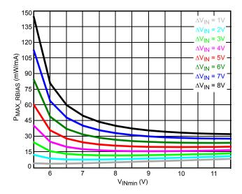
FIGURE 20. NORMALIZED RESISTOR POWER DISSIPATION (AS SELECTED IN FIGURE 17) vs MINIMUM **INPUT VOLTAGE; V<sub>VCC</sub> = 5V**
