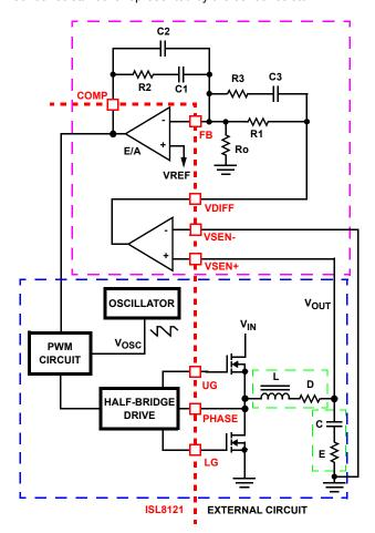
FIGURE 24. VOLTAGE-MODE BUCK CONVERTER COMPENSATION DESIGN
