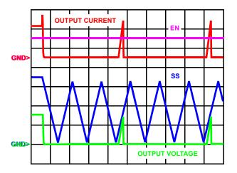
FIGURE 6. OVERCURRENT BEHAVIOR WHILE IN INTERNAL REFERENCE MODE
