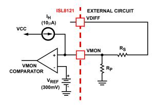
FIGURE 11. SETTING THE MONITORING THRESHOLD AND HYSTERESIS
