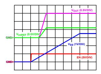
FIGURE 5. NORMAL SOFT-START WAVEFORMS FOR ISL8121-BASED MULTI-PHASE CONVERTER
