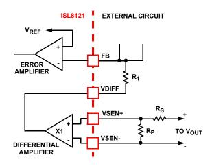
FIGURE 8. SETTING THE OUTPUT VOLTAGE AT THE INPUT
