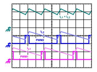
FIGURE 3. PWM AND INDUCTOR-CURRENT WAVEFORMS FOR 2-PHASE CONVERTER
