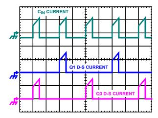
FIGURE 4. INPUT CAPACITOR CURRENT AND INDIVIDUAL
