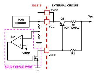
FIGURE 22. INTERNAL SHUNT REGULATOR USE WITH EXTERNAL NPN TRANSISTOR (ACTIVE CONFIGURATION)
