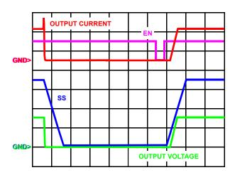
FIGURE 7. OVERCURRENT BEHAVIOR WHILE IN EXTERNAL REFERENCE MODE
